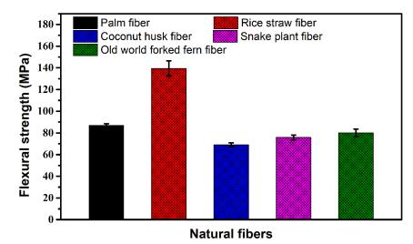
Figure 5. Histogram of the flexural strength of PP composite with different reinforced natural fibers
