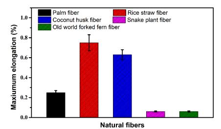
Figure 3. Maximum elongation of PP composite with different reinforced natural fibers
